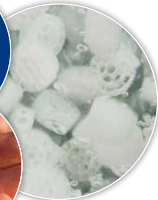
*The core of the process is the biofilm carriers, which are made from polyethylene with a density slightly below of water. Several different types of carriers have been developed in order to optimize their function in different applications.*
