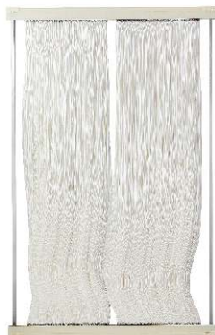
The membranes are grouped in elements each of 5 or 40 m 2
